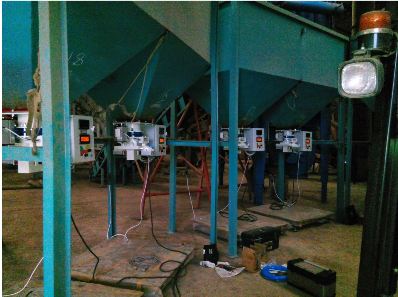
Free Flow Filling Machine application for Mineral Powder
